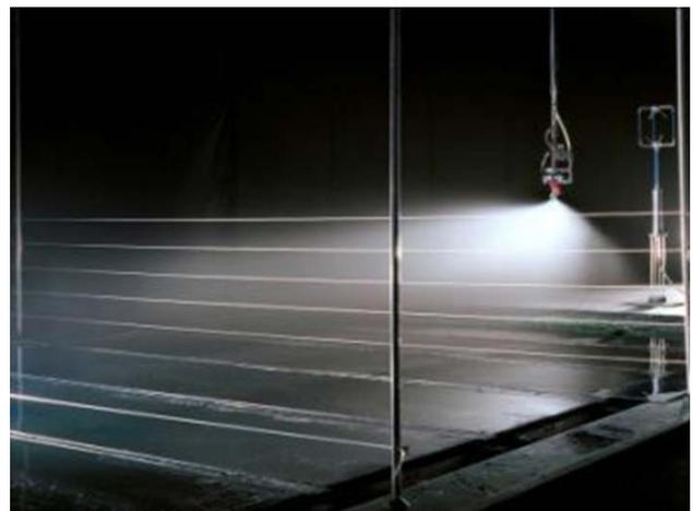
Figure 1 Drift measurement in low speed wind tunnel (UQ)
